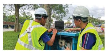
The AguaSMART enables the trigger of early response to potential leakage and preventing water losses
